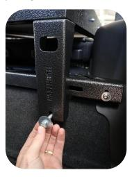
A square nut supplied is placed inside the mounting frame. The frame will hold the nut while you tighten the M8 x 40mm bolt. Do not secure the two/2 slide supports at this point only hand tighten the bolts into place as the slide will need to be positioned.
