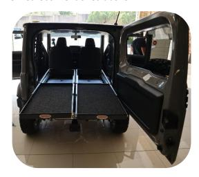
**Note:** An extension shock will need to be installed onto the back door to ensure the door opens wide enough for the slide to open. The extension shock fitment instructions will guide you through the steps needed to replace the back door shock.
