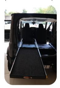
With the use of the remaining M8 x 20mm Bolts and nuts. hand-tighten the slide to the rear mounting bracket.
