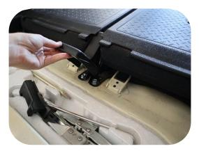
**Pro Tip:** The center plastic cover is also a clip on. Slide your fingers under the cover and pull up until the bottom and top of the cover unclips.
