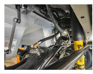
STEP ONE: Pull the factory cap off with pliers and replace with hose section and hose clamps with the brass right angle fitting as shown. (tip; offset the hose clamps and ensure the brass fitting is pushed in all the way)
