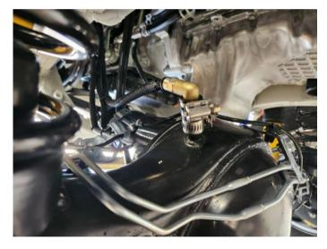
STEP Repeat the step on the other diff. (tip; offset the hose clamps and ensure the brass fitting is pushed in all the way)
