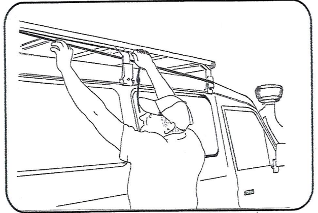
Secure strap provided to your roofrack or bars and then adjust one end by pulling on strap.
