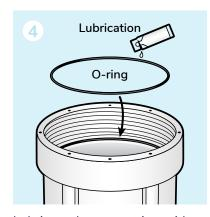
Lubricate the new o-ring with the solution provided, then seat the o-ring in the groove of the housing, as per the instructions supplied. Ensure the o-ring is seated properly.
