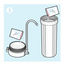
Clean the inside of the housing and base using a food-grade sterilising solution (provided with the replacement cartridge). Thoroughly rinse the housing and base with clean water.
