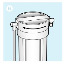
With the system still upside down, screw the base back onto the housing.
