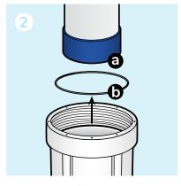
Empty water from the housing and remove (a) the old cartridge and (b) o-ring. Discard both.
