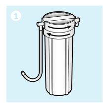
Turn the system upside down and place over a sink, unscrew the base from the housing.
