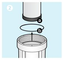
Empty water from the housing and remove (a) the cartridge and (b) o-ring. Discard both.
