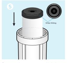
Remove the wrapper and label from the new Doulton Ultracarb Cartridge. Ensure the rubber seals on both ends of the cartridge are seated correctly. Ensure the open end of the cartridge (with the white writing) is facing UP and towards you, then place the cartridge inside the housing. The cartridge can only be installed one way.
