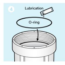
Lubricate the new o-ring with the solution provided, then seat the o-ring in the groove of the housing, as per the instructions supplied. Ensure the o-ring is seated properly.
