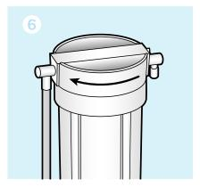
With the system still upside down, screw the base back onto the housing.
