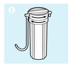
Turn the system upside down and place over a sink, unscrew the base from the housing.
