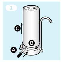
Use the tool supplied with the system, unscrew the outer ring and remove.
