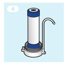
Remove the wrapper and label from the new Hi-Tech Optimiser cartridge. Ensure the rubber seals on both ends of the cartridge are seated correctly, then place the cartridge inside the housing.
