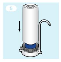
With the cartridge centred in place, put the housing back onto the base ensuring it is sealed on the rubber seal.
