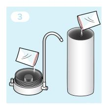
Clean the inside of the housing and base using a food-grade sterilising solution (provided with the replacement cartridge). Thoroughly rinse the housing and base with clean water.
