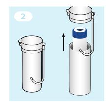
Turn the system upside down and break seal between the housing. Empty water from the housing and remove the base and the old cartridge.
