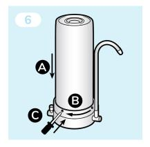
Slide the outer ring back over the housing and tighten down using the tool supplied with the system.
