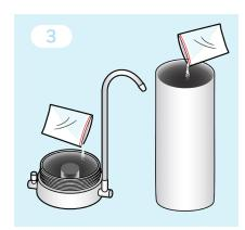
Clean the inside of the housing and base using a food-grade sterilising solution (provided with the replacement cartridge). Thoroughly rinse the housing and base with clean water.
