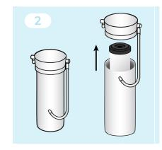
Turn the system upside down and break seal between the housing. Empty water from the housing and remove the base and the old cartridge.
