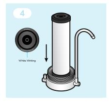
Remove the wrapper and label from the new Doulton Ultracarb Cartridge. Ensure the rubber seals on both ends of the cartridge are seated correctly. Ensure the open end of the cartridge (with the white writing) is facing DOWN and towards base, then place the cartridge on the base. The cartridge can only be installed one way.
