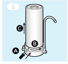
Use the tool supplied with the system, unscrew the outer ring and remove.
