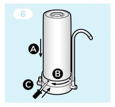
Slide the outer ring back over the housing and tighten down using the tool supplied with the system.
