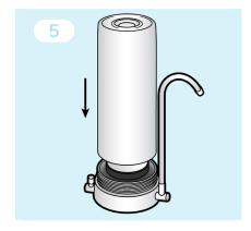
With the cartridge centred in place, put the housing back onto the base ensuring it is sealed on the rubber seal.
