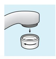
The style of tap you have will determine which of the 3 tap adaptors supplied will be required to attach the diverter to your faucet.
