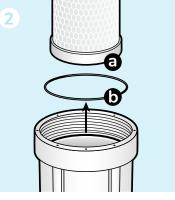
Remove the old filter cartridge (a) and o-ring (b). Discard both.
