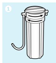
Turn the system upside down and place over a sink, unscrew the base from the housing.
