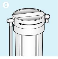
With the system still upside down, screw the base back onto the housing.
