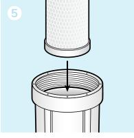
Remove the wrapper and label from the new cartridge. Ensure the rubber seals on both ends of the cartridge are seated correctly, then place the cartridge inside the housing.
