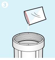
Clean the inside of the housing and base using a food-grade sterilising solution (provided with replacement cartridge). Thoroughly rinse the housing and base with clean water.
