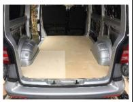
Once fully installed you will have a clean, flat and solid floor to base the rest of your conversion onto.
