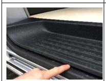
Re-using the original side step will create a gap under the step which needs filled. Better to replace the step with one designed for ply floored vans
