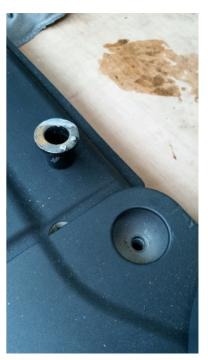
File or drill the rear right-hand seat mounting hole to accept the larger bolt that is supplied in this position.
