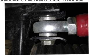
note; please check tightness of spindle pin bolt before use
