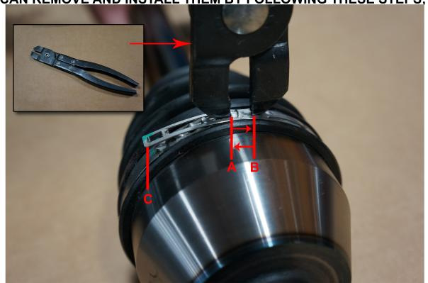
TAKE A PAIR OF PLIERS, WE USE A FLAT TIP PLIER, AND SQUEEZE POINTS A AND B TOGETHER. THIS WILL ALLOW FOR POINT C TO UNLOCK AND THEN THE BAND CAN BE REMOVED.
