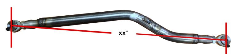
When replacing or installing the rod ends you must measure from the center of one rod end to the center of the other and adjust them accordingly to match the specs listed below.
