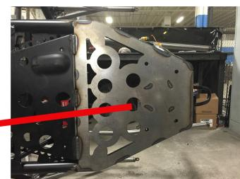
Weld onto front of chassis
