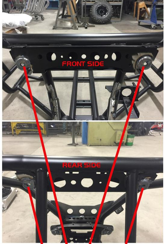
The 4 remaining washers will be used to strenghten the upper shock mount holes. Again you will want to place the washers on the front and backside of the mount and insert the bolt to align the washers. Tac weld the washers in place and then remove the bolt before welding around the outside of the bolt.
