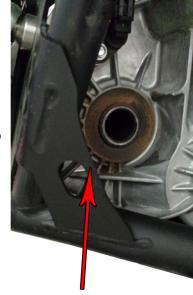
Attention: Due to the larger diameter of the Lone Star Racing heavy duty cv`s, you are required to cut the gusset located on the differential side towards the back of the vehicle. You will want at least I/2" of clearance to allow the cv boot to expand without coming in contact with the gusset.
