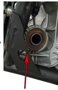
Attention: Due to the larger diameter of the Lone Star Racing heavy duty cv`s, you are required to cut the gusset located on the differential side towards the back of the vehicle. You will want at least I/2" of clearance to allow the cv boot to expand without coming in contact with the gusset.
