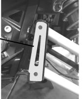
On bolts where #2 is used, you will need to use the supplied Nylon Lock Nuts The gussets are to be placed outside of the a-arm tabs. Picture is for reference only!
