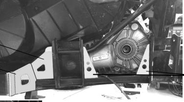
The small triangle gusset welds on top of the rear a-arm mount and welds to the square uprigh tube.
