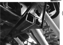
Weld in the 2 1x1 tubes to help strengthen the channel proir to installing the main gusset plate
