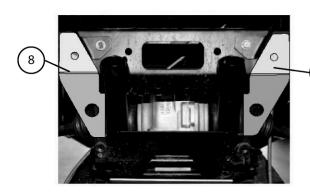
On the rear, first weld on all the a-arm hole supports. You will want to install the bolts throught both plates to ensure the holes stay true to the
