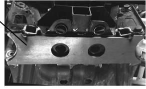
Center the main gusset plate to allow for equal welding on either side.
