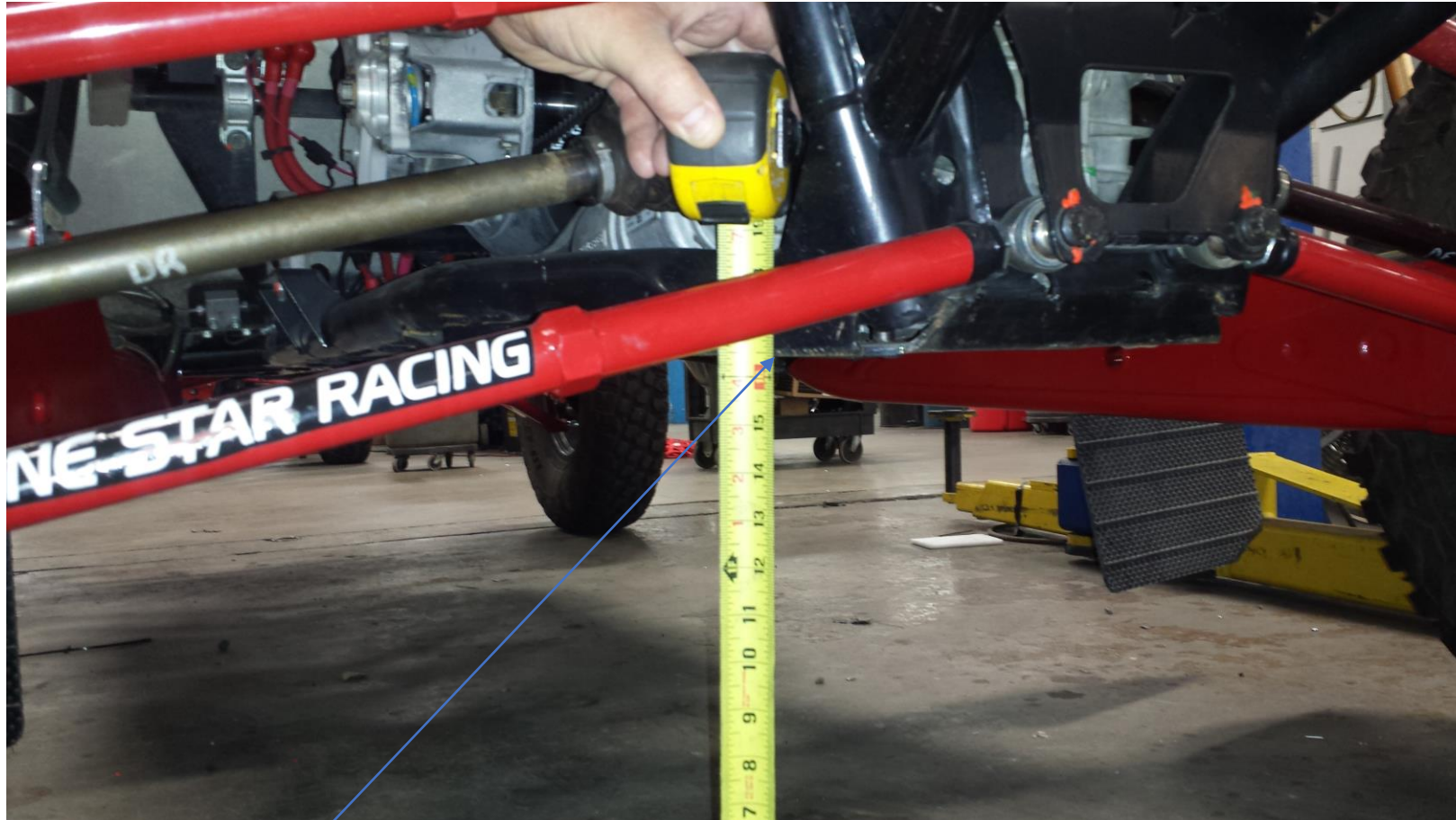
Measuring ride height from this point—in this case just under 16.5"
