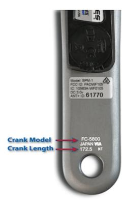
Crank Model Number and Length as seen on a Shimano 5800 left crank arm
