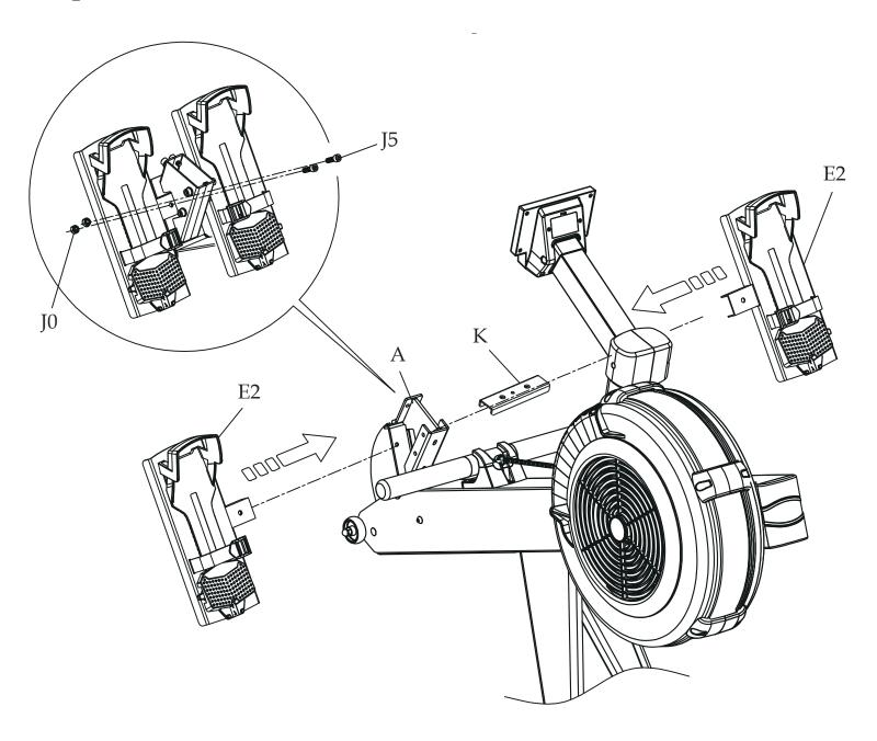
To install foot pedals (E1) and (E2) into (A) Forward Base join the together by Steel Bracket (K). Steel Bracket (K) should slide into place of Foot Pedal (E1). Once placed secure with 2 (J5) bolts and 2 (J0) nuts.
