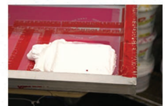
Always keep the image area flooded after printing. This keeps the print from locking up.
