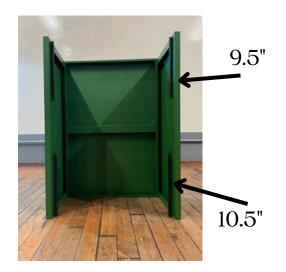
Step 1: Attach Side Panel #2 & #3 to Rear Panel #4. IMPORTANT: Foam facing front. Top of side panels have 9.5" foam & bottom have 10.5" foam. It may be easiest to lay back panel flat on ground when assembling. Aligning 4 screw holes on each side & screw w/ "Assembly Screws".
