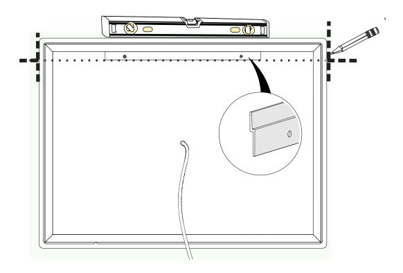
2.Position the aluminum hanging piece precisely over the marked location.Mark these two holes accordingly to ensure accurate alignment and secure installation.
