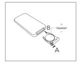
4. Gently push in the holder until securely locked into place.
