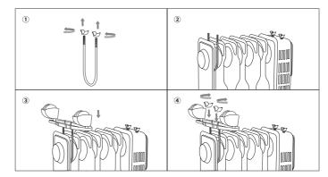
4.Front Casters: Put the other caster mounting plate on the front cover against screws. Screw the wing nuts back to the U-bolt and tighten properly.
