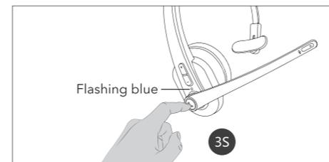
Once connected, the indicator on the Dongle will stay solid blue. The indicator on the headset will flash blue.
