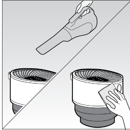
2.Air Outlet: Vacuum up dust with a vacuum cleaner or wipe it with a cloth.
