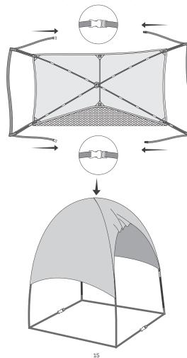
7. Insert two ends of the linked short pole into the sleeves in the middle of the tent cloth edges to prop up the tent top.
