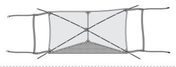
5. Insert the ends of each pole into the respective sleeves on the belts attached to the four corners of the tent cloth. The tent cloth will be stretched taut.
