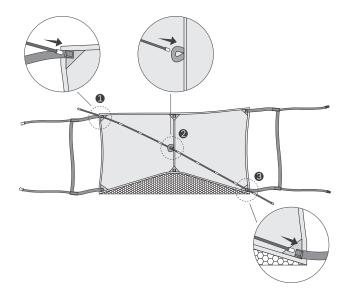
4. Repeat the previous step for the other long pole, make the two long poles cross in the middle of the tent cloth, forming an "X" shape.
