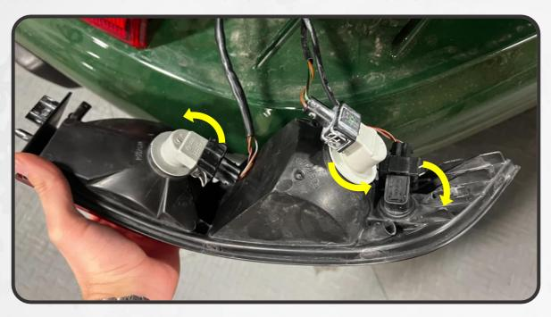
4. UNPLUG THE THREE BULB SOCKETS FROM THE HARNESS BY PINCHING THE METAL CLIPS ON THE SIDES OF THE CONNECTOR AND PULLING. INSTALL ONE OF THE BLOCK-OFF PLUGS ONTO THE SIDE MARKER BULB (CIRCLED BELOW)
