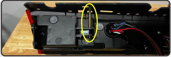
18. CONNECT THE CENTER TAIL LIGHT CONNECTOR (YELLOW) TO THE NEW CENTER TAIL LIGHT ASSEMBLY. IF YOU HAVE A U.S. SPEC CAR (NO REAR FOG LIGHTS), CONNECT IT TO THE CONNECTOR LABELED "US". IF YOU HAVE A EURO SPEC CAR (EQUIPPED WITH REAR FOG LIGHTS), CONNECT TO THE CONNECTOR LABELED "EU". CONNECT YOUR BOOS BAR AS WELL IF INSTALLED (RED)
