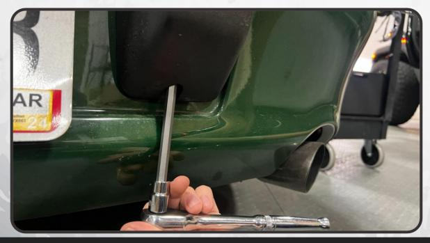
13. REMOVE THE GROMMET LOCATED ON THE TOP OF THE BUMPER COVER ABOVE THE LICENSE PLATE
