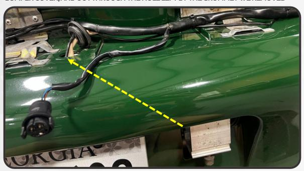
16. PULL THE WIRE THROUGH THE GROMMET AND REINSERT THE GROMMET INTO THE HOLE
