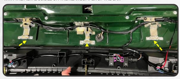
20. FIT THE CENTER TAIL LIGHT ONTO THE CAR, ENSURING THAT THE 3 TABS SLOT INTO THE METAL GUIDES. REINSTALL THE THREE 4MM ALLEN SCREWS (YELLOW) AND TIGHTEN DOWN THE THREE FLATHEAD MOUNTING PINS (RED)
