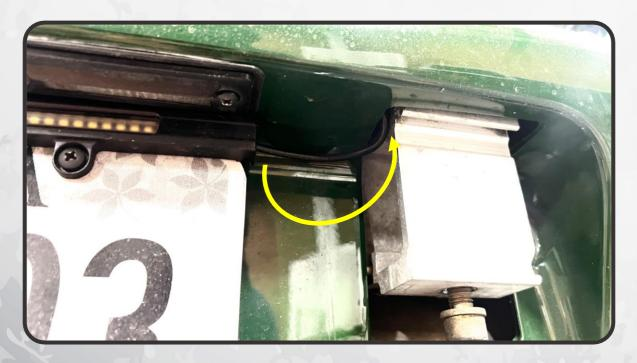
15. ROUTE THE BOOST BAR WIRE FROM THE HOLE BEHIND THE BUMPERETTE, BEHIND THE BUMPER COVER, AND OUTTHROUGH THE HOLE LEFT BY THE GROMMET WE REMOVED
