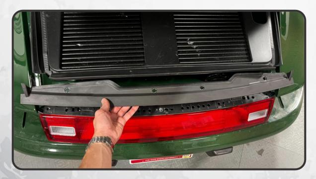
8. UNSCREW THE 3X 4MM ALLEN SCREWS (YELLOW) SECURING THE CENTER TAIL LIGHT TO THE CAR, AND LOOSEN THE 3 PHILLIPS HEAD MOUNTING PINS (RED)
