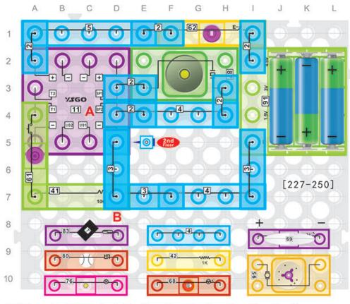
227.Press Switch Controls the Sounds of Machine Guns from the Buzzer Build the circuit, press the switch[62], if you press the press switch[61], you will hear the sounds of machine guns from the buzzer[87].
