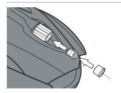
1. Insert the battery pack into the rear of the Rollsys® system, with the green PCB board facing outwards.
