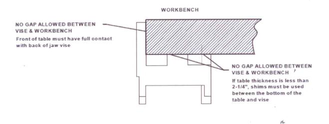
Figure 1: Mount Back Jaw Casting to Work Bench
