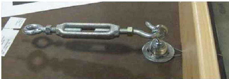
UNDERSIDE OF TABLE SHOWN FOR TURNBUCKLE ASSEMBLY
