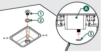
Install the Gas/Water Fixtures 2 by placing them into the pre-drilled holes on the top surface. Secure them using the Washers 4 and Lock Nut 5.
