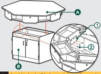
Double check all bolts are tightened securely before use. Check all bolts periodically. Failure to completely tighten the bolts may result in tipping and possible injury!
