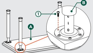
If a screw is difficult to secure tightly, uninstall the screw and carefully deepen the predrilled hole slightly, using the correct size drill bit.
