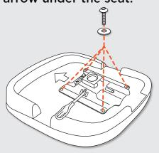
Hand tighten all screws and then tighten them completely using the allen wrench.
