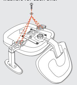
Hand tighten all screws and then tighten them completely using the allen wrench.
