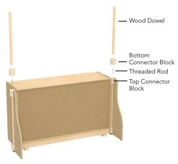
4. Screw in the provided threaded rod so 1½" sticks out of the top connector block. Place the bottom connector block over the threaded rod and screw on the wood dowel until tight. Repeat for other side.
