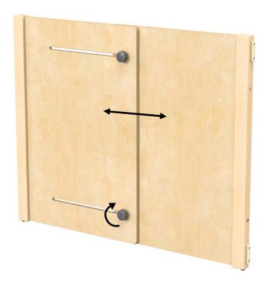
Slide Accordion Panel to desired length. Tighten knobs to lock Panel into place by turning knobs clockwise (about 1½ full rotations). Follow instructions on page 9 to attach an Accordion Panel to other KYDZ Suite items and page 11 to attach to Jonti-Craft furniture items.
