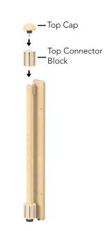
2. Next, replace the top connector block and screw in the top cap.
