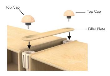
Place the Filler Plate over the top connector blocks. Reinsert the top caps and tighten.
