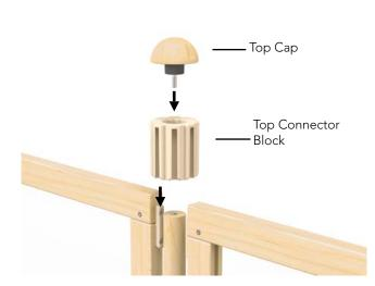
4. Replace the top connector block by aligning the Hub Connector Tabs on the two Panels with the grooves and the post with the connector block Screw in the top cap until tight.
