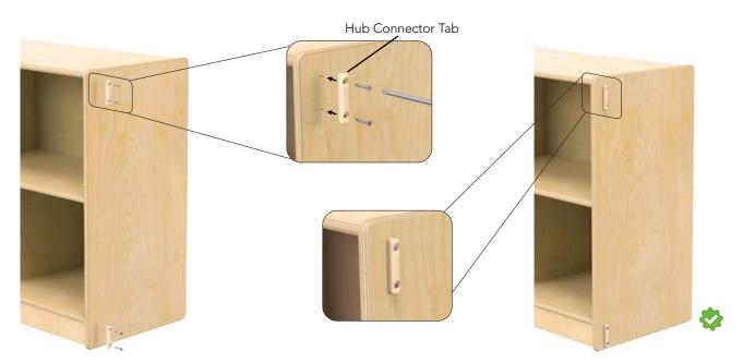
3. Attach the Hub Connector Tabs by inserting two #6 - 34" flat head screws (supplied) through the holes in each tab and into the drilled holes of the Jonti-Craft furniture item. Tighten using a medium Phillips head screw driver.
