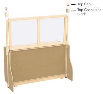
6. Place the top connector blocks over the Hub Connector Tabs on the Panel and screw in the top cap from the Hubs.
