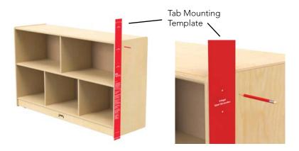
1. To apply Hub Connector Tabs to a Jonti-Craft furniture item, first place the Tab Mounting Template included in your starter kit on the side of the unit as shown. Depending on where the tabs are to be placed, align the edge of the template with the front or rear edge of the furniture item. Mark the holes for the appropriate height Hub Connector Tabs needed. Remove the template and set aside.
