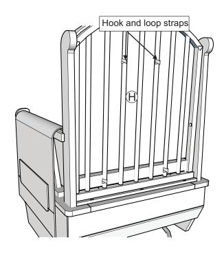
Attach back cushion (G) to back rest (D) with hook and loop straps.
