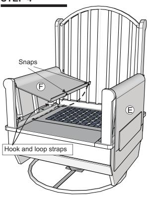
Attach arm rest cushions (E & F) to arm rests (B & C) with hook and loop straps then snap to base.
