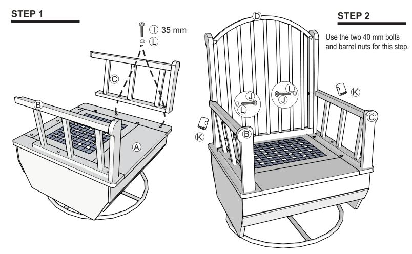
Attach right arm rest (C) to base (A) using two washers (L) and bolts 35 mm (I). Tighten with allen wrench (M). Keep bolts loose until back rest is attached.
