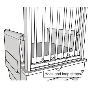
Attach seat cushion (G) to back rest (D) with hook and loop straps.
