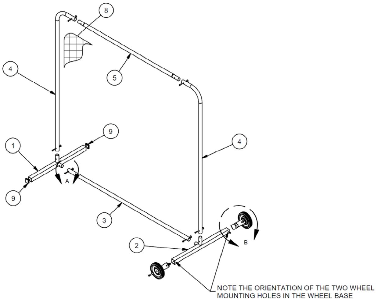
Figure 2 Wheel Orientation
