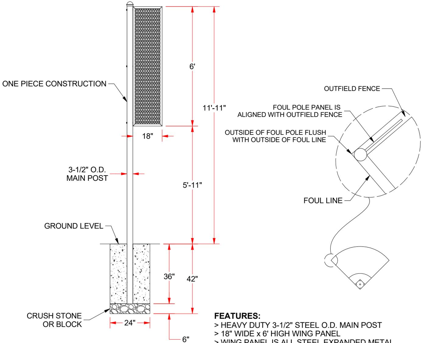
\* MANUFACTURER RECOMMENDS THE FOOTING BE REINFORCED WITH 6 PIECES OF 3/4" REBAR.
