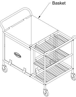
Step #7 - Install the basket as shown (with the Angeles emblem facing out) using the hook and loop fasteners sewn onto the cloth.
