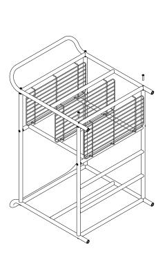
Step #5 - Carefully work the tabs of the middle wire shelf into the holes of the End being careful not to allow the tabs of the top shelf work out. Repeat again for the bottom shelf and install the remaining bottom two screws. *TIGHTEN ALL SCREWS TIGHT.*
