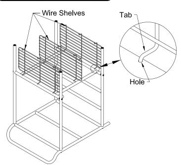
Step #3 - Turn the assembly on end and install the tabs on all three wire shelves into the holes of the Upright.
