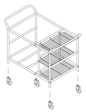
Step #6 - Install the four casters by screwing one into each leg.
