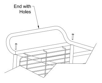
Step #4 - Carefully place the tabs of the top wire shelf into the holes of the End and install ONLY the top two screws.
