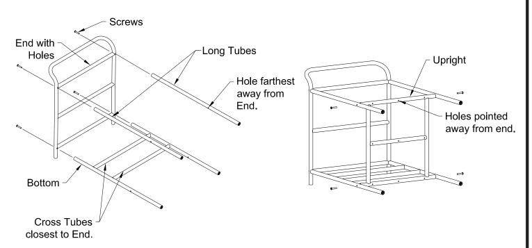
Step #1 - Assemble the End with the Long Tubes (hole farthest away from End) and the Bottom (the cross tubes closest to the end) as shown. **DO NOT TIGHTEN SCREWS DOWN TIGHT!**
