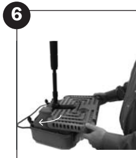
6 Place the Lid around the Nozzle and on top of the Filter Pad.
