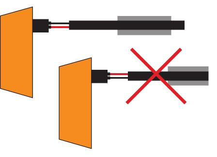
Move the adhesive-lined heat shrink over the connector so that it mounts completely over the top of the connector.
