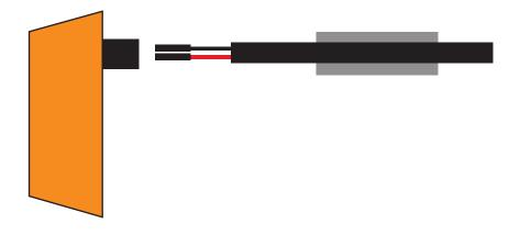
Plug the female wire terminals into the male terminals on the inside of the connector using caution not to bend the male terminals. Red (+) goes on the inside, black (-) towards the edge of the light fixture as pictured.
