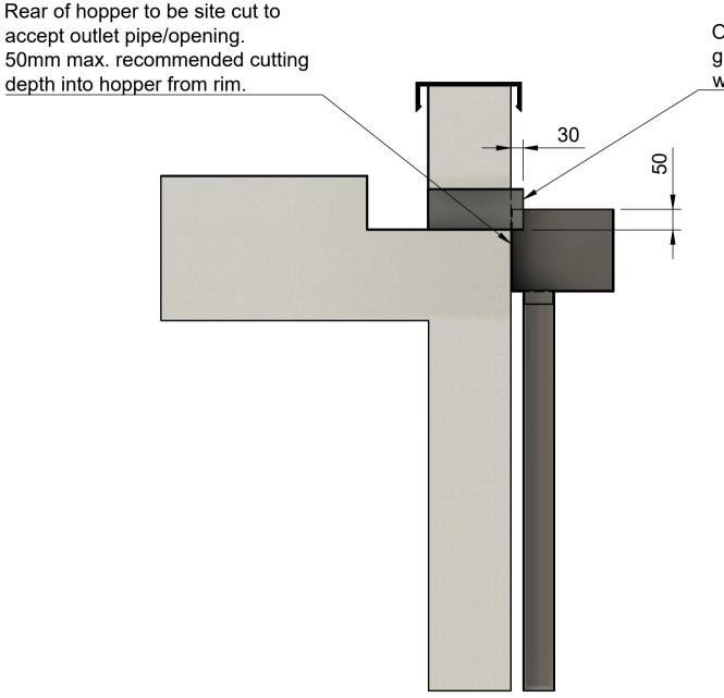
Outlet pipe/opening from internal gutter to project 30mm past wall face.
