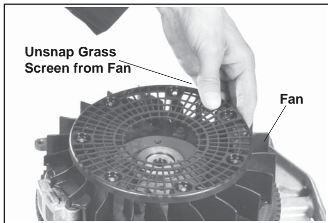
Figure 9-32. Removing Plastic Grass Screen.
