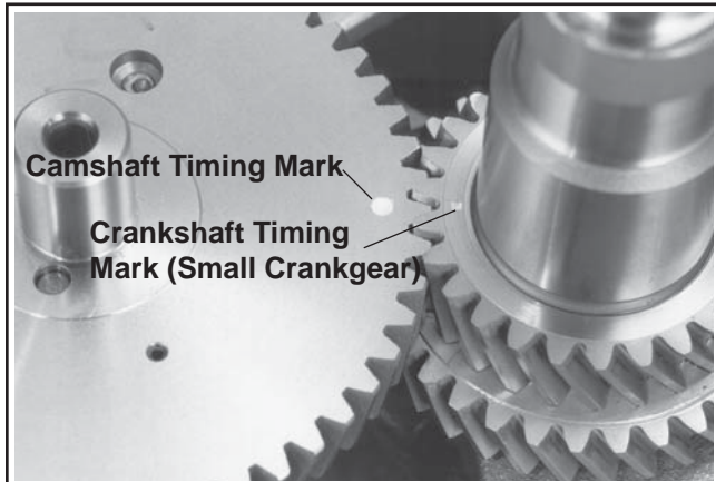
Figure 11-13. Aligning Timing Marks on Crank Gear and Cam Gear.
