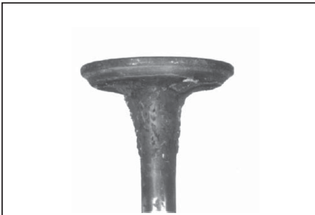
Gum: Gum deposits usually result from using stale gasoline. This condition is often noted in applications where fuel is not treated with stabilizer or drained out of tank during the off season. Gum is a prevalent cause of valve sticking. The cure is to ream the valve guides and clean or replace the valves, depending on their condition.
