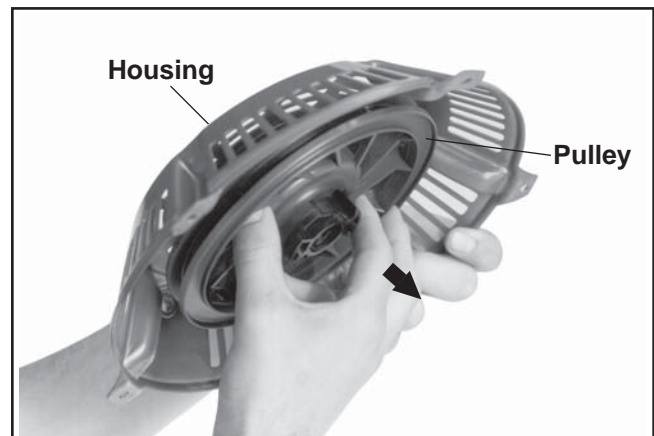
Figure 7-7. Removing Pulley from Housing.
