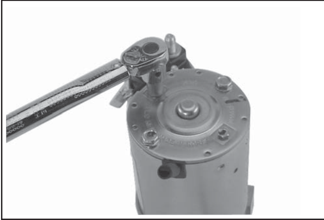
Figure 8-65. Torquing Brush Holder Screws.
