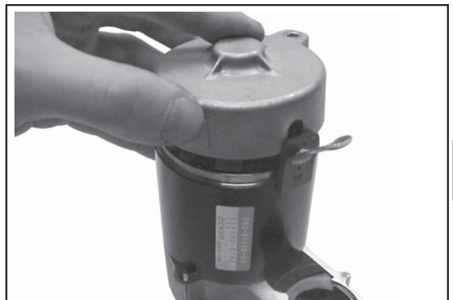
Figure 8-34. Installing End Cap.
