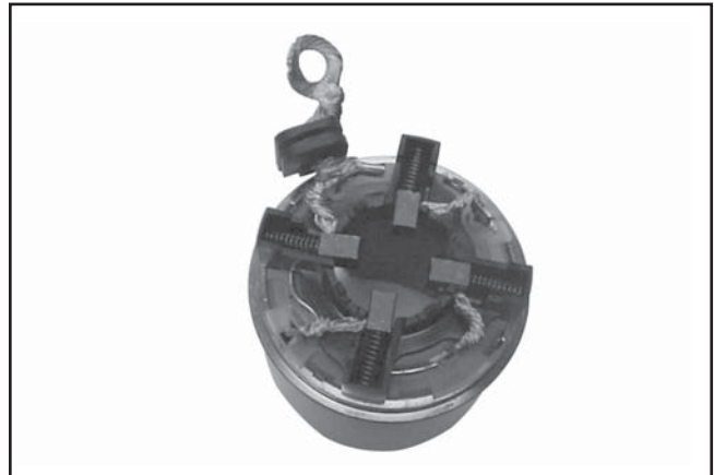
Figure 8-30. Mounting Brush Holder to Frame.
