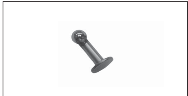
Figure 11-35. Tappet and Ball Bearing Welded Together.
