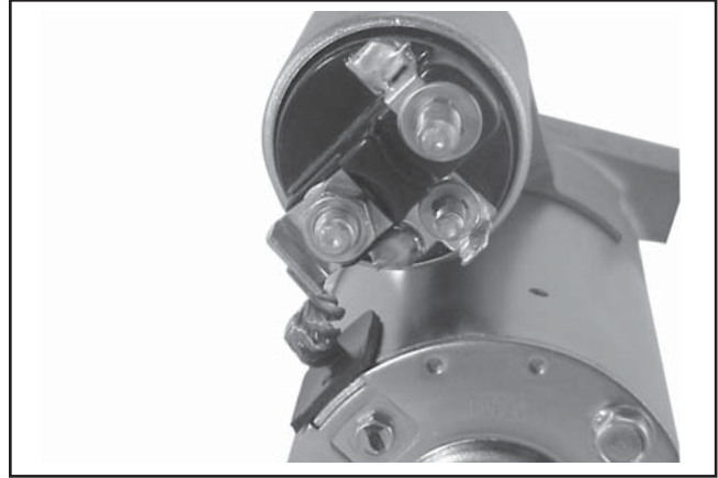
Figure 8-67. Positive Brush Lead Connection.
