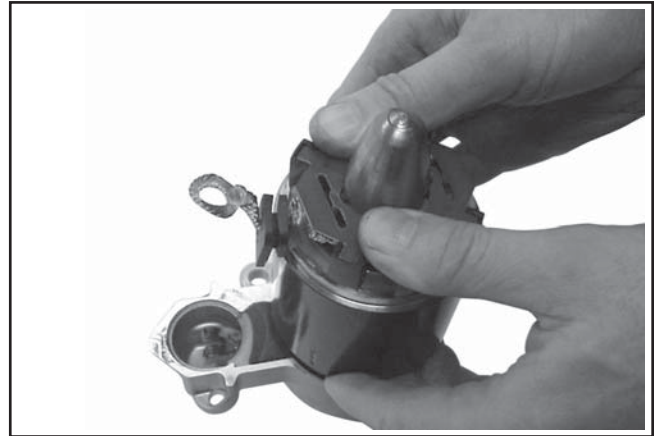
Figure 8-33. Installing Frame with Brush Plate Assembly.
