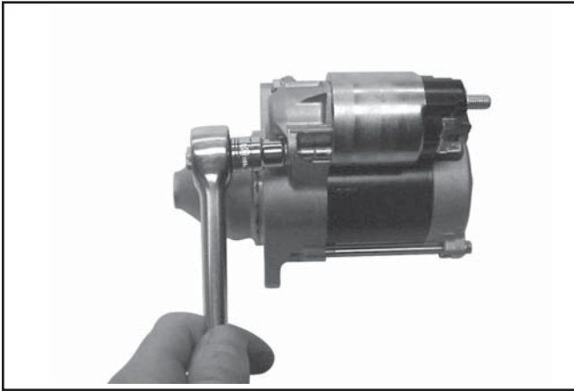
Figure 8-35. Installing Thru Bolts.
