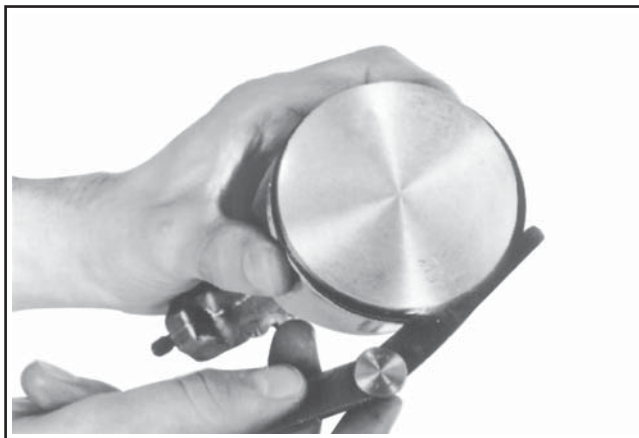
Figure 10-9. Measuring Piston Ring Side Clearance.
