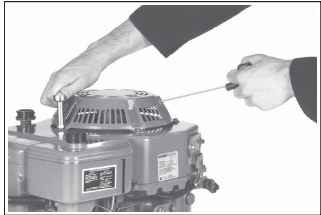
Figure 11-70. Installing Retractable Starter.
