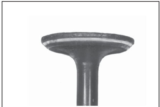
Overheating: An exhaust valve subject to overheating will have a dark discoloration in the area above the valve guide. Worn guides and faulty valve springs may cause this condition. Also check for clogged air intake, and blocked fins when this condition is noted.
