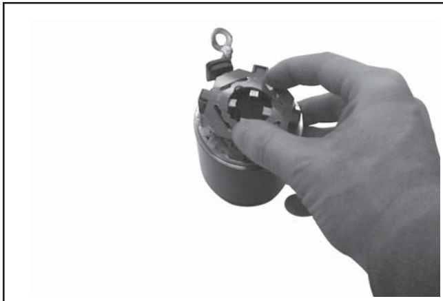
Figure 8-31. Holding Insulator in Place.
