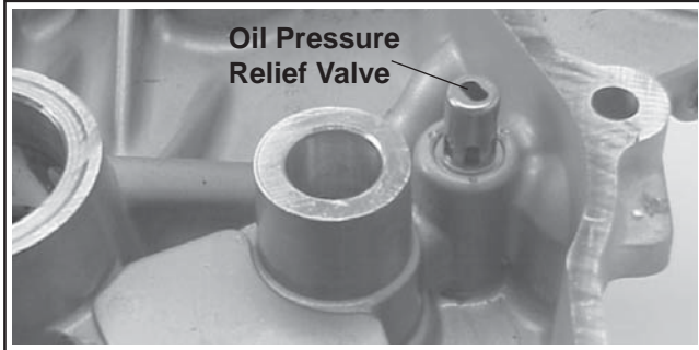
Figure 6-8. Oil Pressure Relief Valve Styles.
