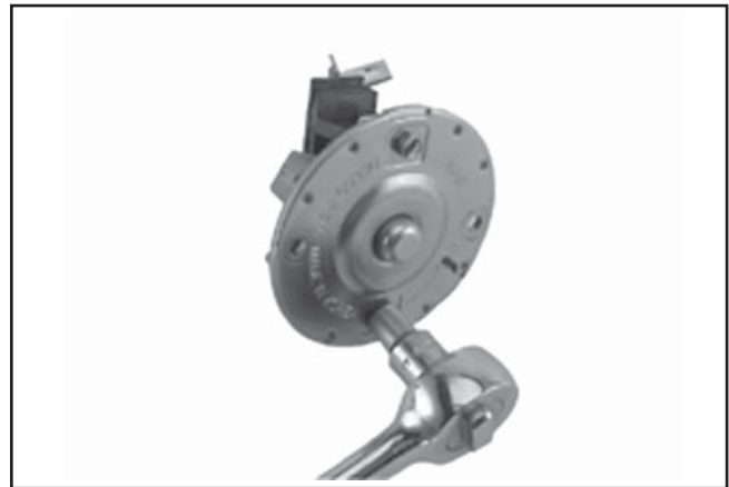
Figure 8-52. Removing Brush Holder.
