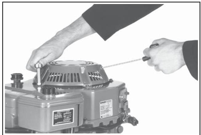
Figure 7-2. Installing Retractable Starter.
