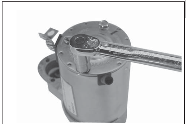
Figure 8-64. Torquing Thru Bolts.
