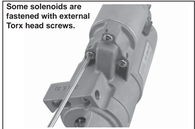
Figure 8-38. Removing Solenoid Screws.
