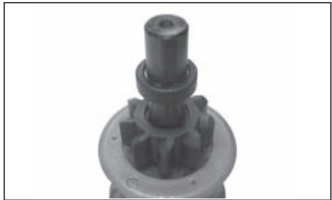
Figure 8-20. Lock Collar around Retaining Ring.
