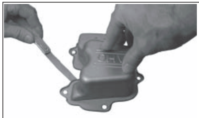
Figure 10-11. Checking with Feeler Gauge.
