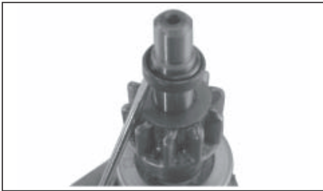
Figure 8-45. Installing Stop Collar/Retainer.
