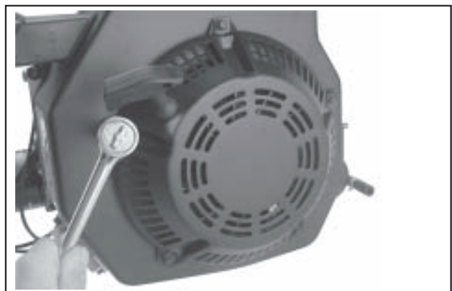
Figure 7-2. Removing Retractable Starter.
