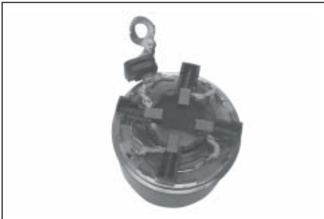
Figure 8-22. Mounting Brush Holder to Frame.
