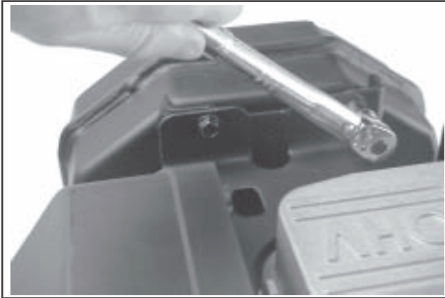
Figure 11-63. Installing Upper Muffler Bracket and Mounting Screws.
