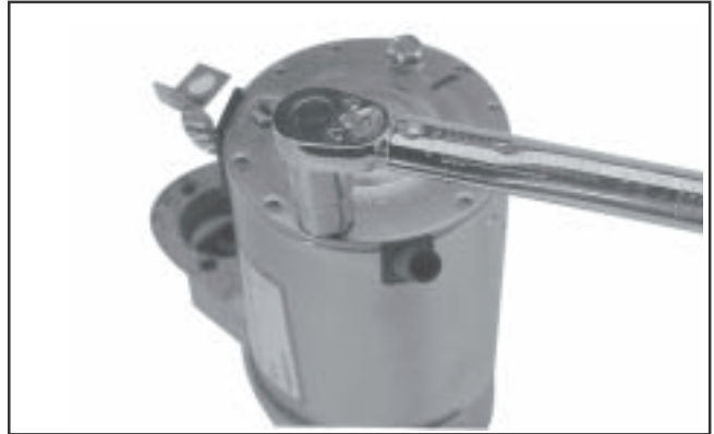
Figure 8-55. Torquing Thru Bolts.
