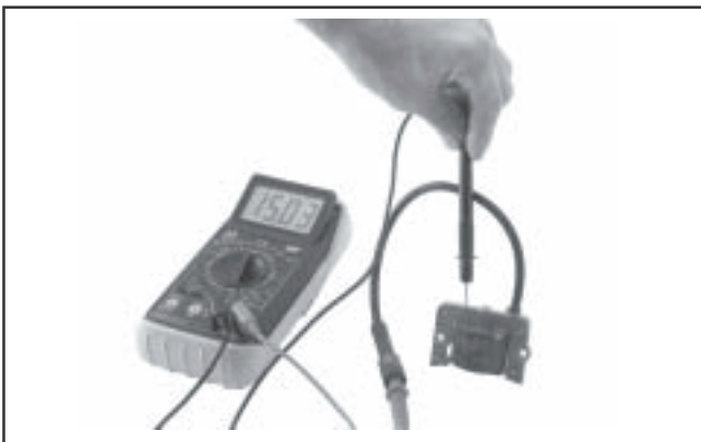
Figure 8-4. Testing Module Secondary.
