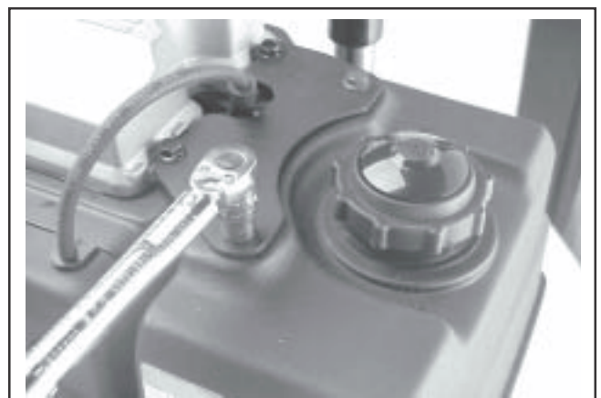
Figure 11-50. Installing Fuel Tank Upper Mounting Screws.
