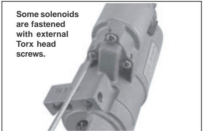
Figure 8-30. Removing Solenoid Screws.
