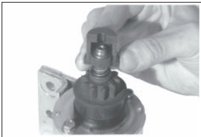
Figure 8-14. Assembling Larger Inner Half Around Spring Retainer.
