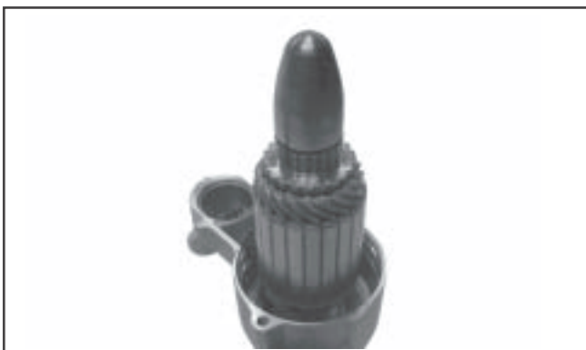
Figure 8-24. Tool on end of Armature.
