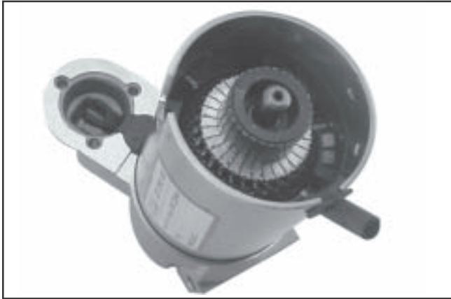
Figure 8-49. Installing Frame and Drain Tube.
