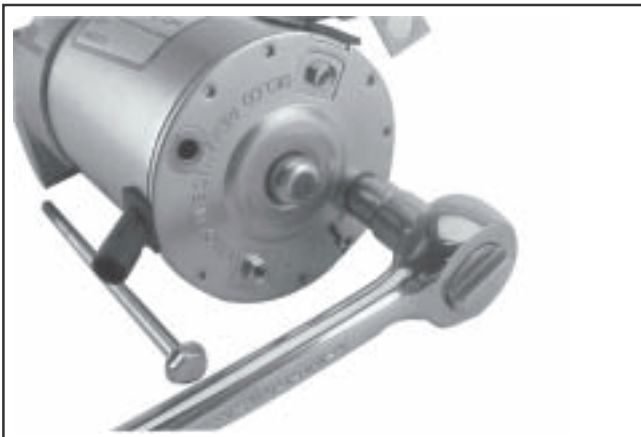
Figure 8-33. Removing Thru Bolts.
