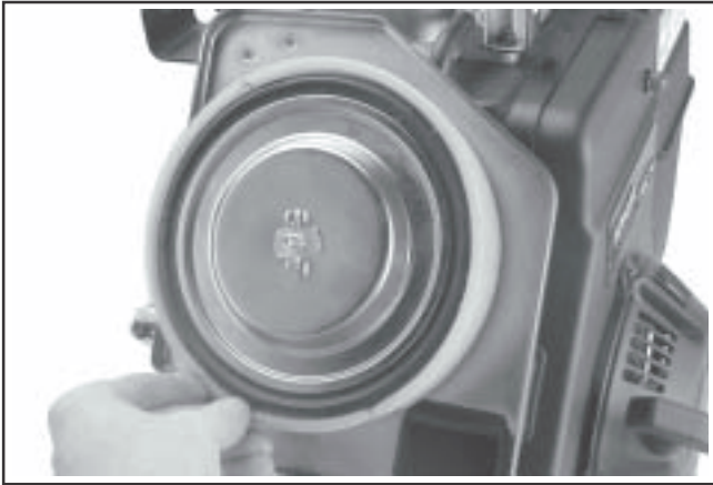
Figure 11-59. Installing Air Cleaner.
