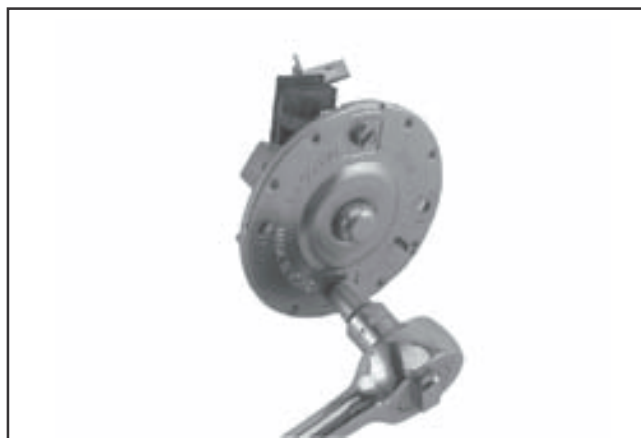
Figure 8-43. Removing Brush Holder.
