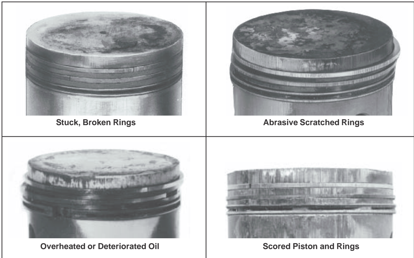
Figure 10-5. Common Types of Piston and Ring Damage.
