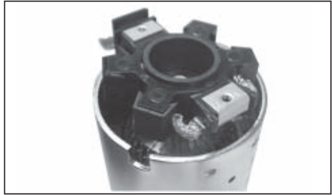
Figure 8-51. Installing Brush Holder Assembly with Supplied Tube.
