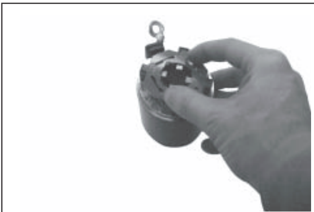
Figure 8-23. Holding Insulator in Place.
