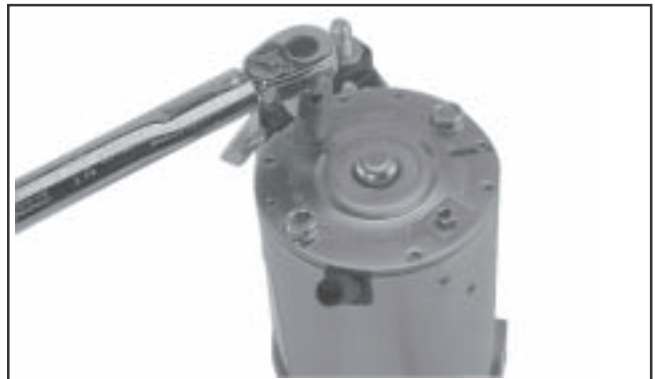
Figure 8-56. Torquing Brush Holder Screws.
