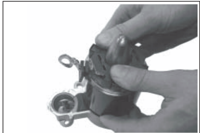
Figure 8-25. Installing Frame with Brush Plate Assembly.
