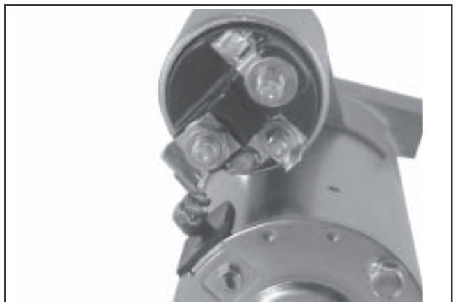
Figure 8-57. Positive (+) Brush Lead Connection.
