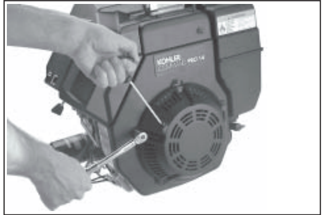
Figure 11-61. Installing Retractable Starter.
