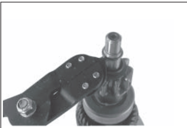
Figure 8-39. Removing Retaining Ring.
