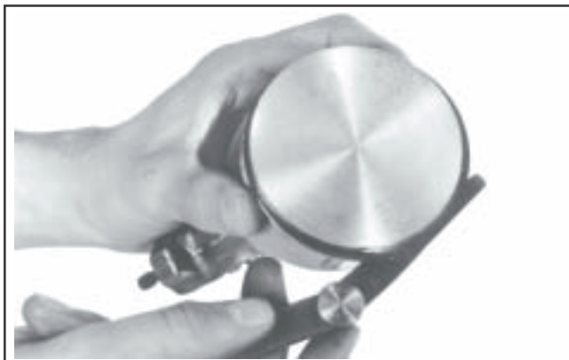
Figure 10-7. Measuring Piston Ring Side Clearance.
