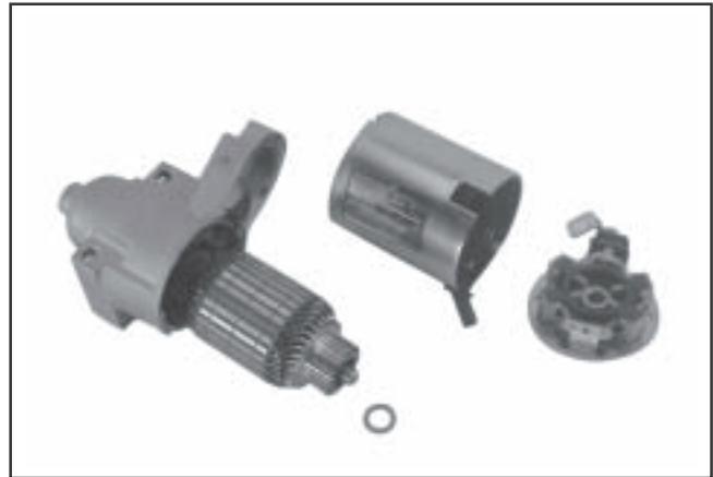
Figure 8-35. Starter Frame Removed.
