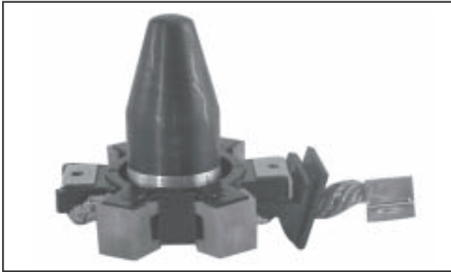
Figure 8-53. Brush Installation Tool with Extension.
