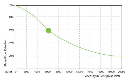
During the conveyance of a fluid with a viscosity of 6000cPs, the pump rate decreases to 60% of its rated value (100% = water). Valid for 3/4" pumps & larger.
