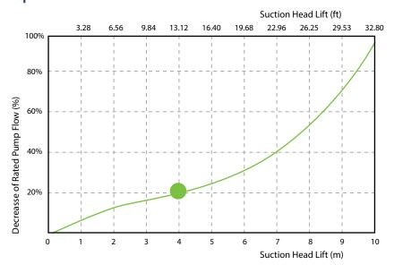
With a suction lift of 4m, pump rate decreases by approximately 20%. Valid for pumps 3/4" and larger; data varies with pump configuration.
