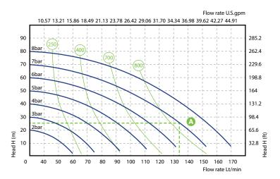
At performance point **A**, the pump will require approximately 7 bar air inlet pressure. To arrive at this figure, follow the solid blue curve to the left to read the air pressure rating in BAR.
