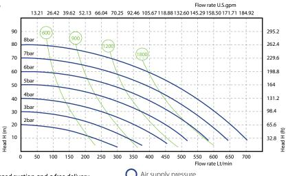
The curves and performance values refer to pumps with submerged suction and a free delivery outlet with water at 20°C, and vary according to the construction material.
