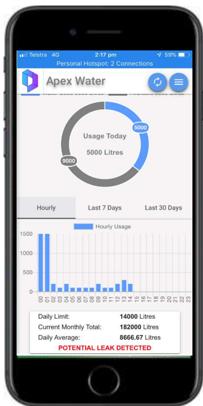
Leak detection alert
