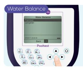
Water Balance can be set to use the Palintest Scale or Langelier Index. Select the preferred option and press OK
