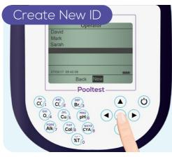
To create a new Operator ID or Sample ID, scroll to the bottom of the list, then select 'New' to create an ID.
