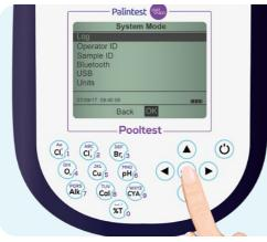
To access Operator ID or Sample ID from the main menu select 'System Mode' then 'Operator ID' or 'Sample ID'.
