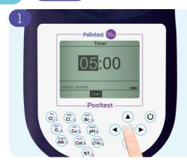
A timer can be set after the blanking process. Refer to the test method to see if this is required. The development time for the test will automatically appear. This can be modified using the arrow keys. Press start to set timer running.
