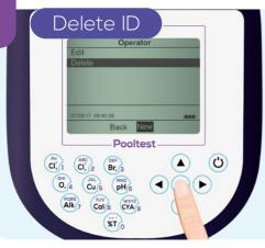
To delete an Operator ID or Sample ID, highlight the option, and select 'Delete.
