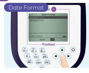
To change the date format select 'System Mode' from the main menu then 'Date Format' DD/MM/ YYYY or MM/DD/YYYY.
