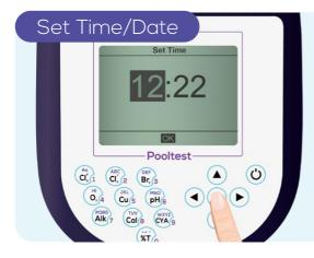
From the main menu select 'System mode' then 'Set Time' or 'Set Date'. Use the navigation keys to select and adjust each part of the time or date.
