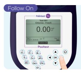
Refer to the test method to see if this is required. If a follow-on test is available, it will appear in the bottom menu. Select if required.
