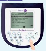
When the instrument starts up it will display the **'Choose a Test'** screen.
