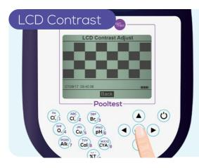
From the main menu select 'System mode' then 'LCD Contrast'. The LCD screen contrast can be manually adjusted. Use the up/down buttons to adjust the contrast until the alternating shapes are clearly visible and press 'Saye'.
