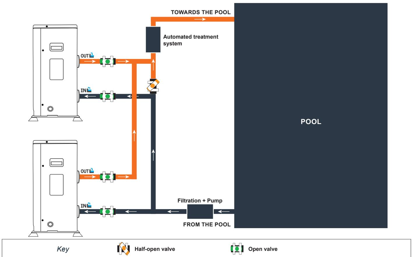
The filter located upstream of the heat pump must be regularly cleared so that the water in the system is clean, thus avoiding the operational problems associated with dirt or clogging in the filter.
