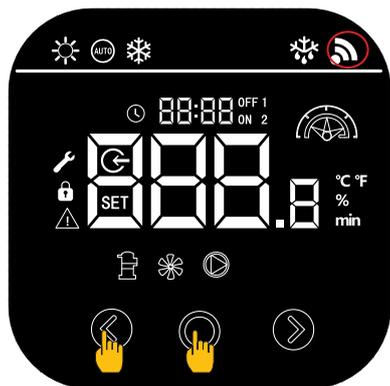
Press + simultaneously for 5s, flashes quickly, the control box is ready to be paired.
